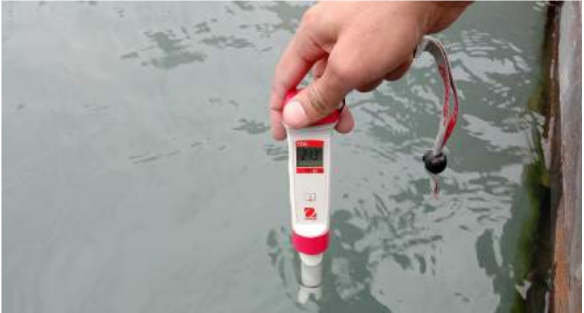
Photograph 35: Testing of Lake Water with Portable TDS Meter
